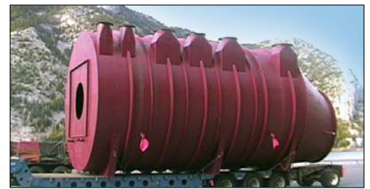
Coal Fines Fired Heater
